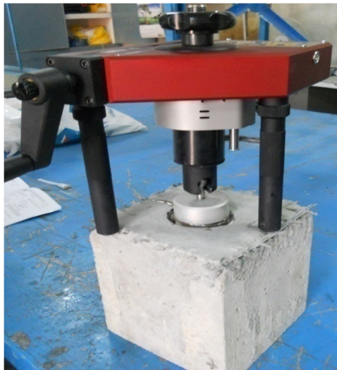
Figure 3.21 Pull-off test on FABcrete
