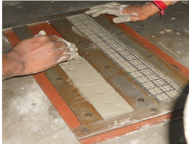
Figure 4.3 Casting of specimens
