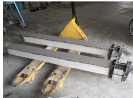
FABcrete strengthened beams
